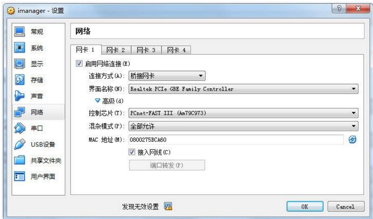
Note: Click the Refresh button after the MAC address to update it. Select the physical network card of the machine, not the virtual network card for the interface name
